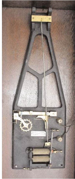
Figure 9: Movement with iron backplate. Pendulum removed to show crutch clearly. Total height 455mm. Private collection.
