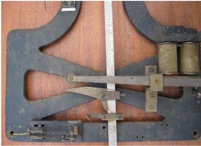
Figure 6 (above): 'Murday type' master in unrestored condition.
