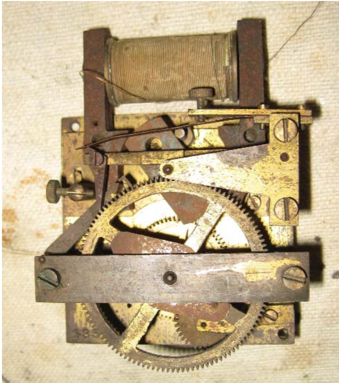
Figure 12. Murday style 'silent' slave movement (rear view).
