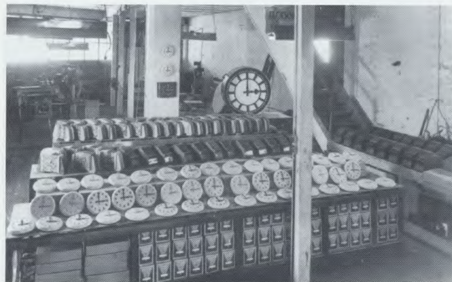
Australian Clocks circa 1956. Underneath the table are Enfield chiming movements to be fitted to Sydney made wooden cases (Oxford Cabinets) visible behind and at the right. The white painted spun aluminium dials housed Smiths synchronous mains movements. The large double dial (with impulse movement) probably went to Innisfail, Queensland.
