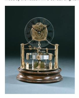
It differs from the two discussed above in having a polished steel balance wheel with weights rather than the simple lead wheel. The support for the wheel-work and upper bearing for the balance wheel arbor are different too, although such differences are also seen in the 'normal' electromechanical version.
