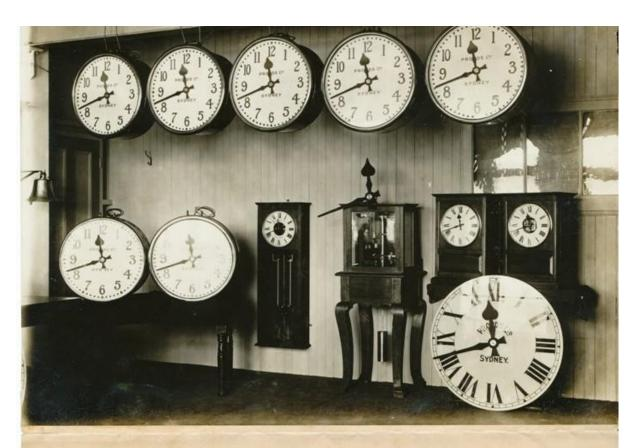
Some of the special electric self-contained clocks made to the order of the Sydney Harbor Trust, and installed on the various Ferry Jetties, Circular Quay.
