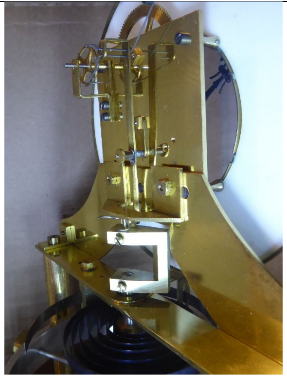
The serial number on the clockwork module is covered by the mounting bracket.
