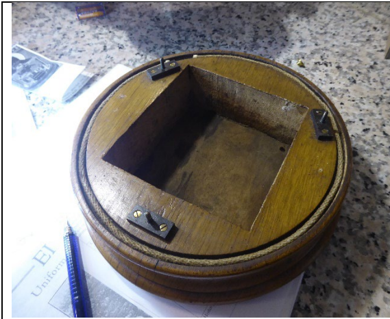
The clock is held on the wooden base by three knurled nuts
