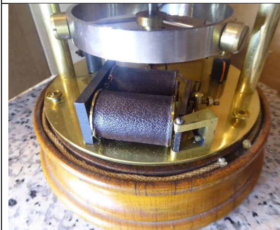
The armature is pivoted rather than being mounted on a flexure
