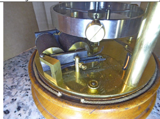
The armature has a return spring
