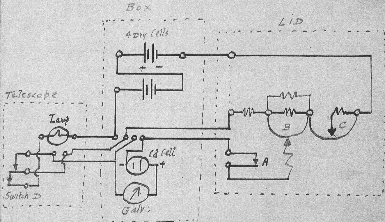
Turning large knob, both contacts B and C move, Key D being closed.
